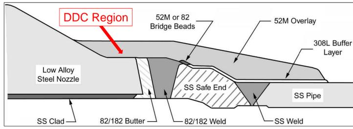
Figure 1: Schematic of multipass weld used in nuclear industry with DDC-susceptible region marked (52M Overlay) [1].
