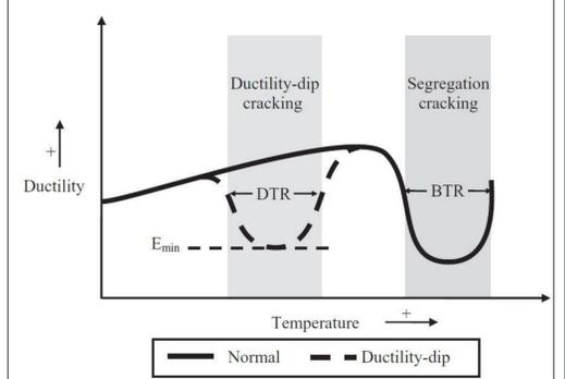
Figure 2: Ductility vs. temperature graph for a material prone to DDC [2].
