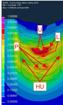
Figure 3: Cumulative plastic strain map in Sysweld FEA model showing approximate crack category locations.
