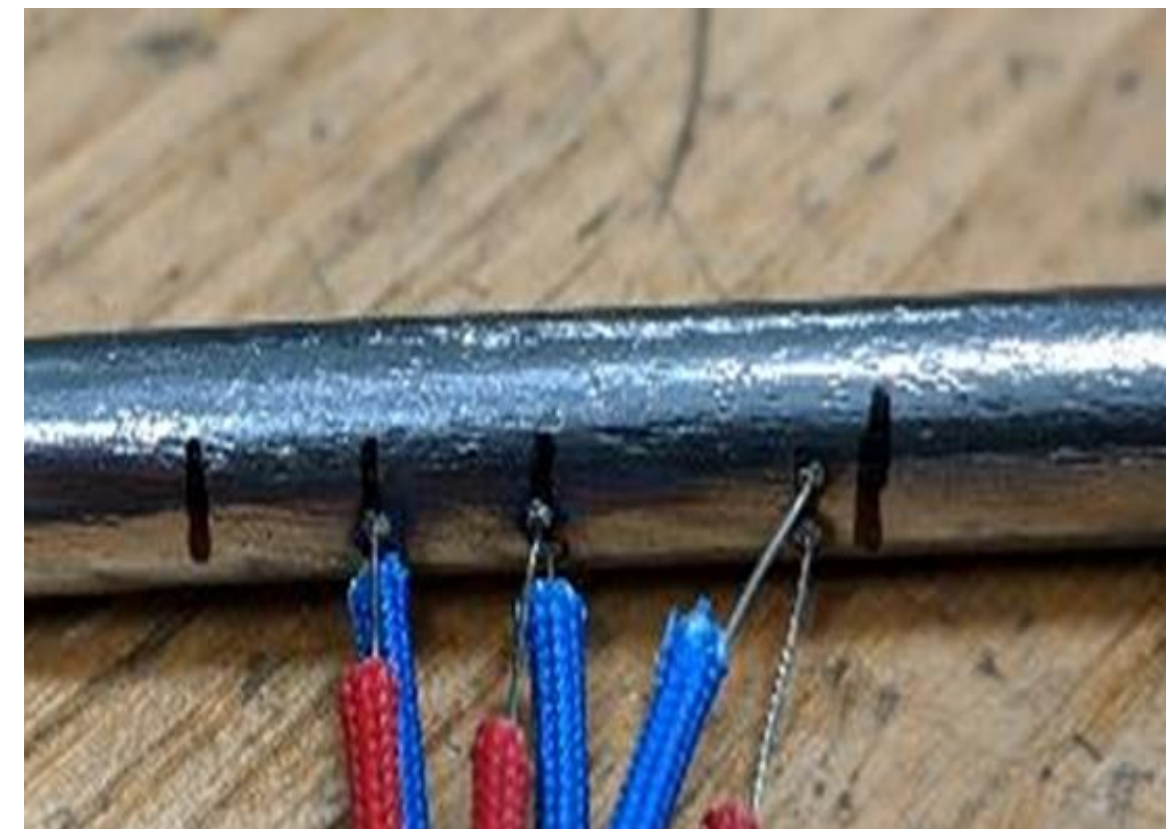
A gleeble sample with thermocouples attached.
