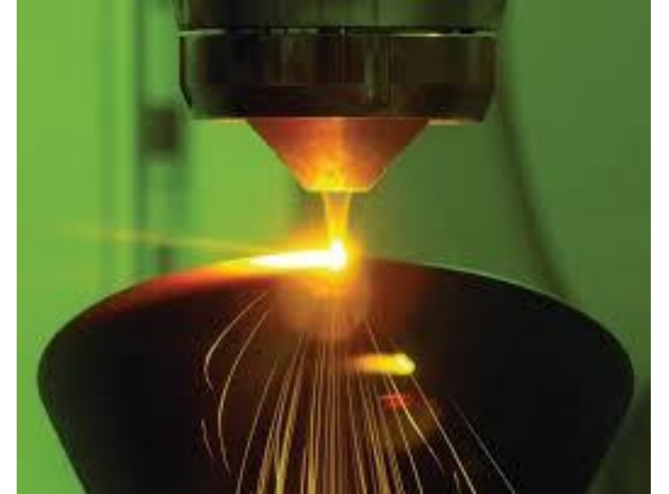
Example of real-world application of laser-based additive manufacturing (Henry Royce Institute, 2020)
