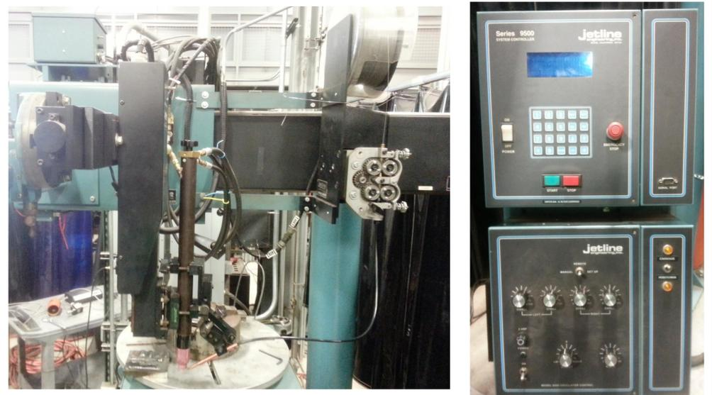
Jetline cold wire TIG machine (left) and controller (right)
