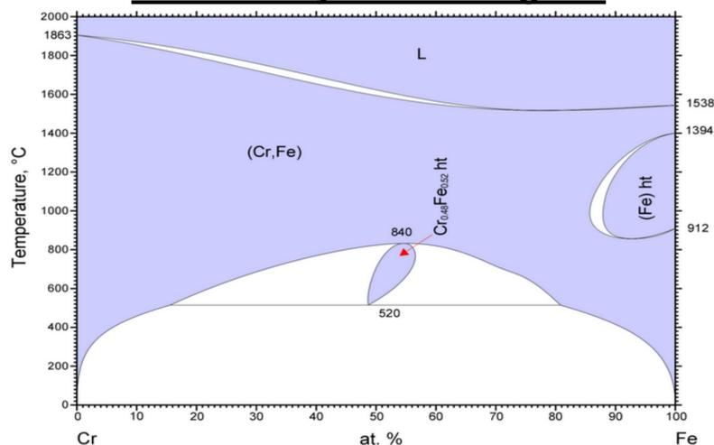
In the phase diagram above, the sigma phase formation range is indicated its molecular formula  $(Cr_{0.48}Fe_{0.52})$
