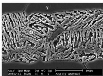
2 Sigma phase precipitation inside ferrite on gauge length of creep sample of 316L steel tested at 550°C for 85 000 h with load of 150 MPa; etchant - V2A Beize, SEM
