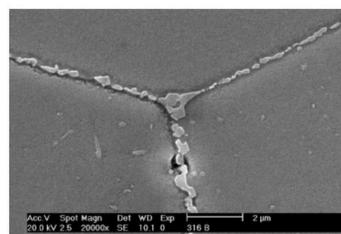
3 Sigma phase precipitation at grain boundaries on gauge length of creep samples of 316L steel tested at 550°C for 85 000 h with load of 150 MPa (SEM); etchant - V2A Beize
